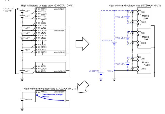
The individual cell voltages in the example given in Figure 1 are only about 2 V, but a common mode voltage of up to 600 VDC may be applied if 300 ch of cells are connected in series. When measuring for a high voltage application like this, please use the high withstand voltage type (GX90XA-10-V1) which can handle a common mode voltage of up to 600 VACrms/VDC.
